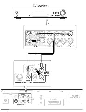
The diagram shows standard video connections, but you can alternatively use the S-Video or component video connections if they're available.
